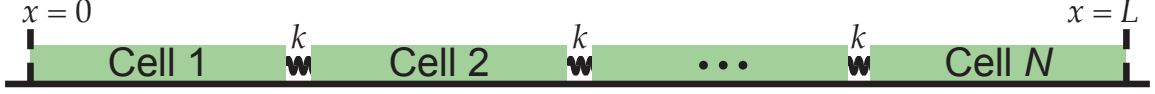
Figure 8.7: Minimal one-dimensional picture of N cells adhering via cadherin-based adhesions, modeled as linear springs of stiffness k .
