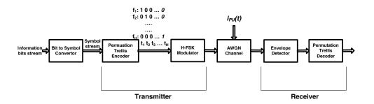
Fig. 2: Signal processing from transmitter to receiver
