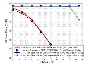
Fig. 4: Performance of PTC based MFSK and Conv. codes under narrowband PU interference.
