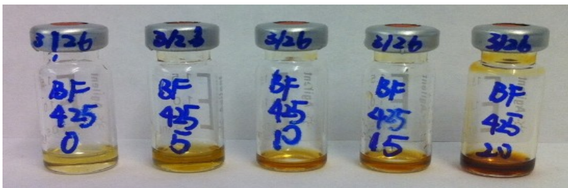
(iii). Temperature: 425°C; Times: 3, 8, 13, 18 and 23 minutes (from left to right)
