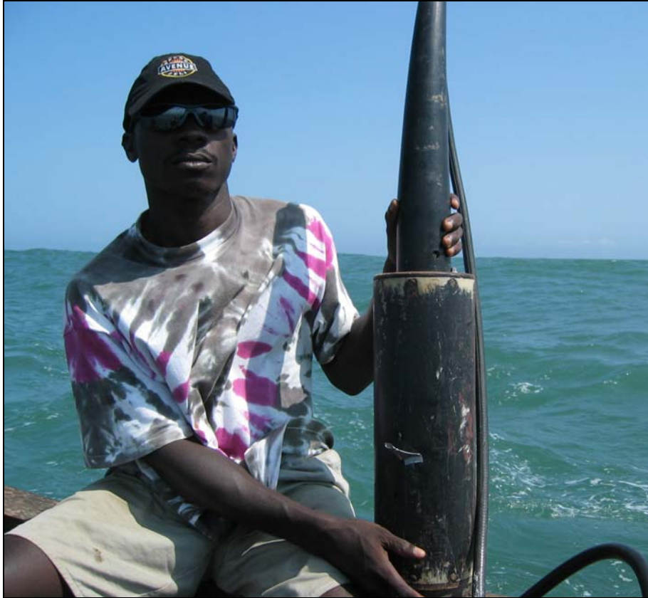
Figure 5.8 Survey assistant Isaac Abban holding the EG&G 866 magnetometer sensor. Photograph by G. Cook.
