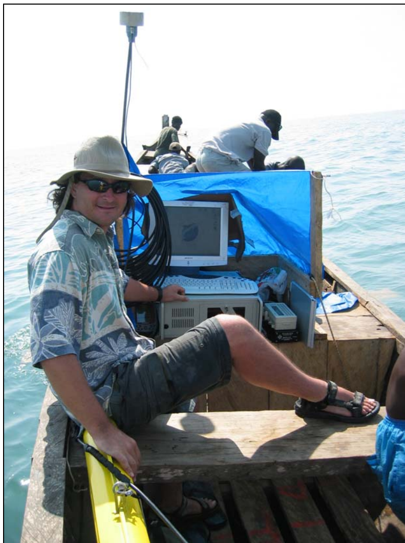
Figure 5.7 The survey setup during 2003 field work. The author is in front of the desktop computer running the sonar software, with the sonar “fish” by his right hand and GPS antennae behind him. Photograph by Michael Tuttle.
