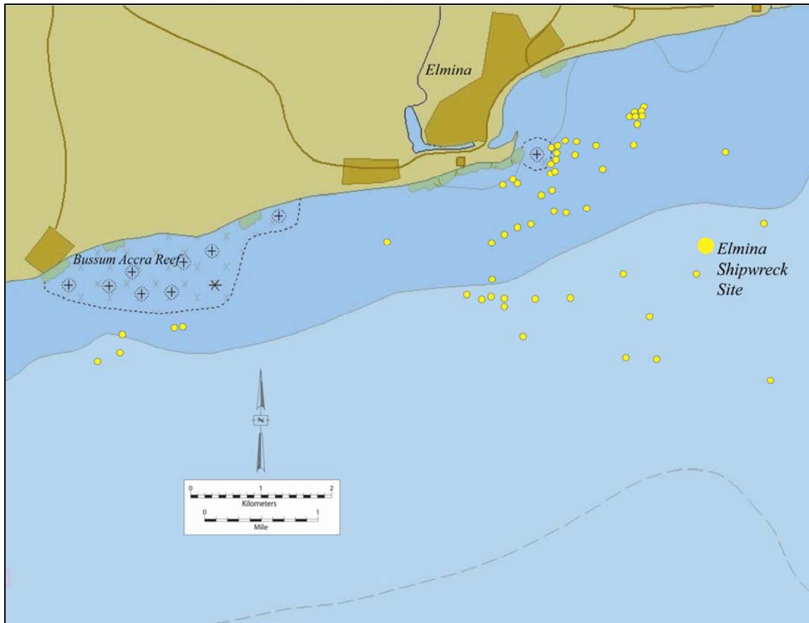
Figure 5.11 Plot of sonar targets resulting from the 2003 survey. Map by G. Cook using digital British Admiralty Chart 3113.
