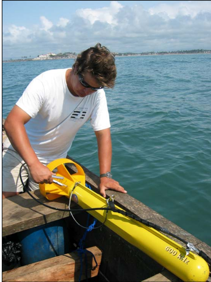
Figure 5.9 Michael Tuttle preparing the side scan sonar fish for survey. Photograph by G. Cook.
