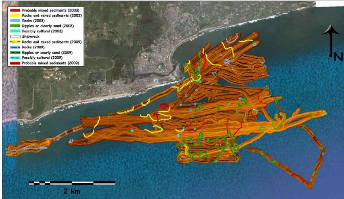
Figure 7.8 Mosaic showing side-scan sonar coverage combining the 2003 and 2009 surveys (After Horlings 2011: 147).
