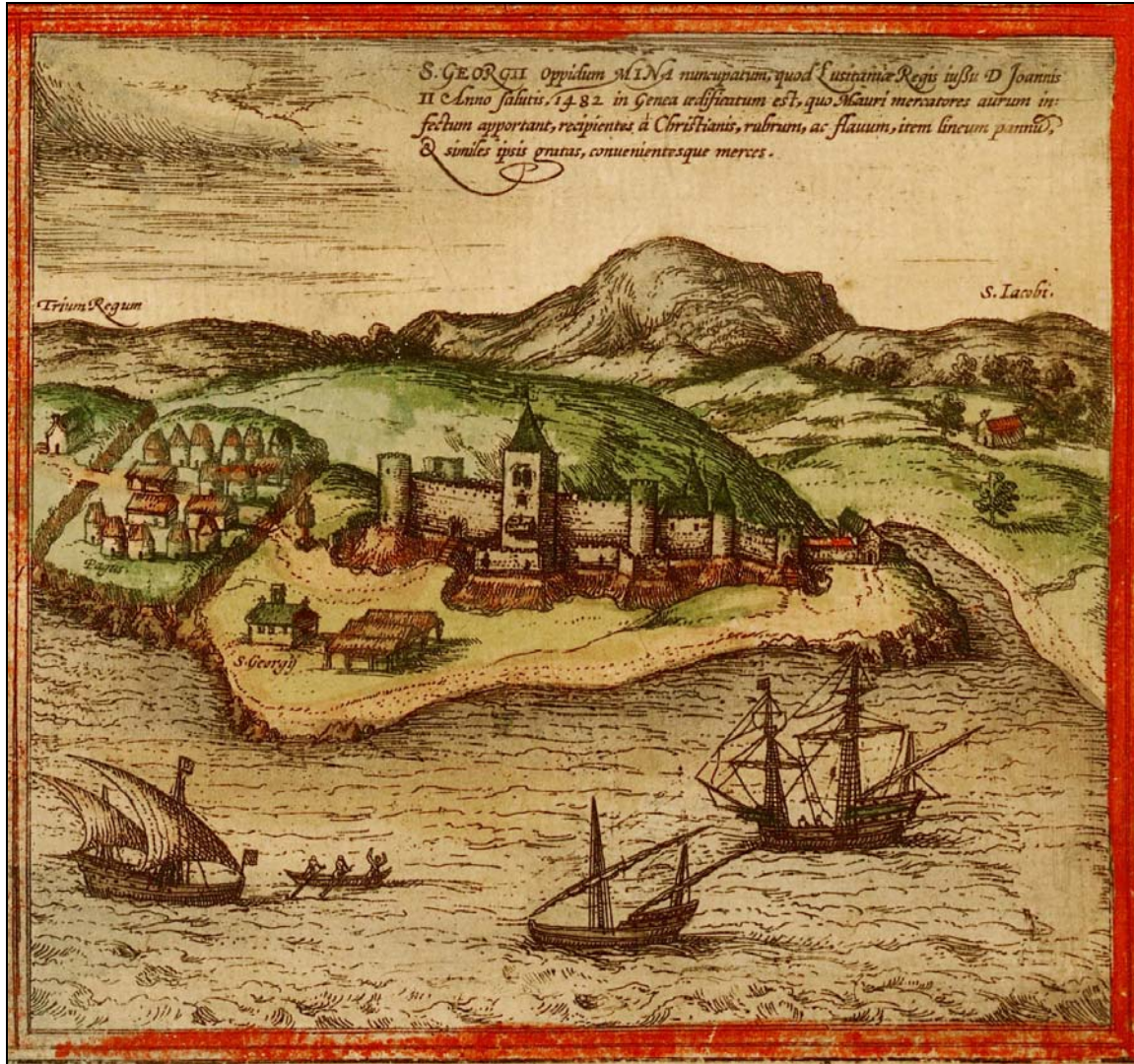
Figure 4.3 Sixteenth-century ships offshore of Elmina. In this image, vessels are shown sailing and at anchor offshore of the Castle. The characteristics of the smaller vessels, notably the multiple masts, lack of a forecastle and low sterncastle, are suggestive of caravels . The larger vessel, with square sails on the main and fore mast, lateen sail on the mizzen mast, and large fore and sterncastles, is indicative of the nao (Braun and Hogenberg 1990: plate XXIX).
