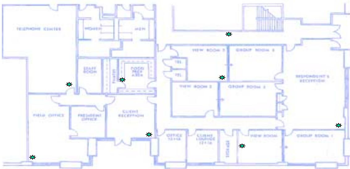
Fig. 1. Four storey building layout with wireless sensors
