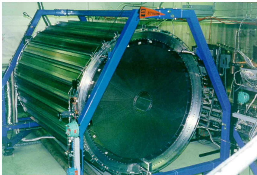
Fig. 24. Photograph of Outer Cylinder during construction, supported on the A-Frame, with “dummy panels” in place.
