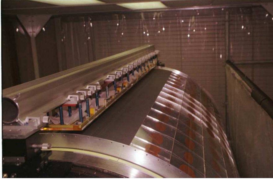
Fig. 22. Photograph of one row of crystal radiators being aligned on the inner carbon fiber cylinder. Previously epoxied rows are shown on the right half of the cylinder. The inner half of the end flange is visible in the forefront.
