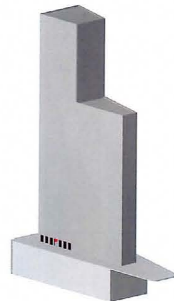
EXTERIOR SHEER WALLS
