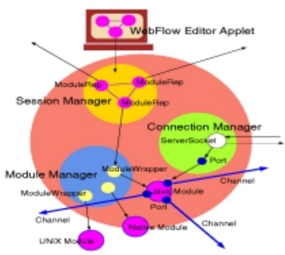
Figure 20: Architecture of the WebFlow server: includes Java servlet based Session, Module and Connection Managers responsible for interacting with front-end users, backend modules and other WebFlow servers in the middleware.
