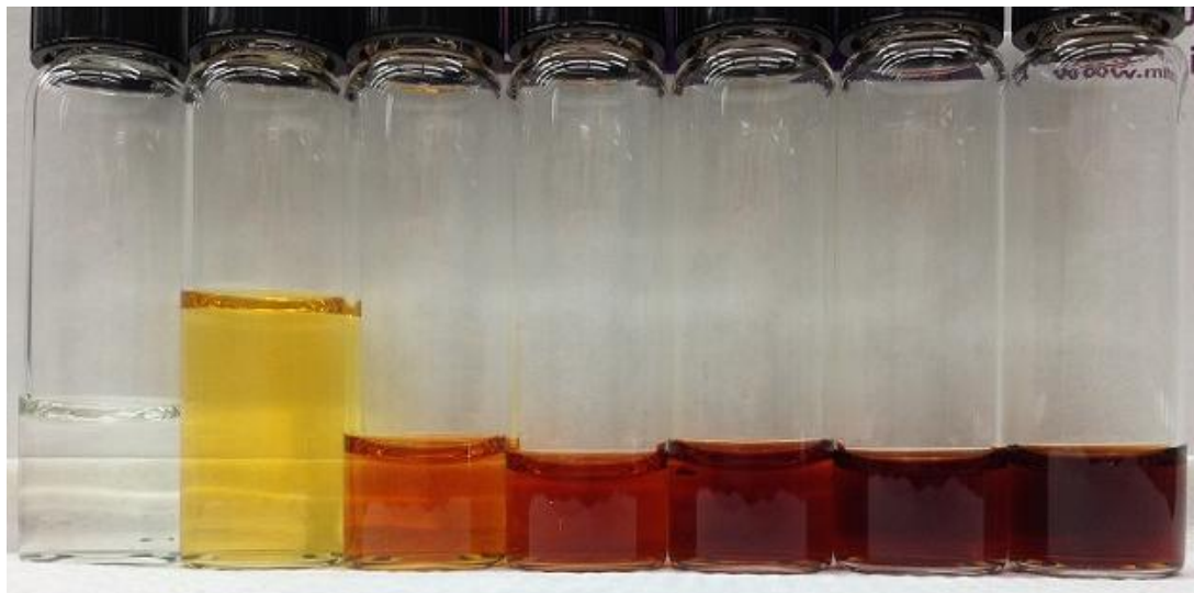
Figure 5-7: Browning of the TMX along the timeline of preparing the stock. From left to right, aliquots were taken from 0 min to 120 min in 20 min interval. 100 mM of each of the three reactants were used.
