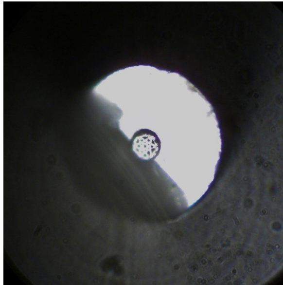
Figure 4.3 Sample A - SSF with a one-scale hexaflake unit (magnification: 400x)
