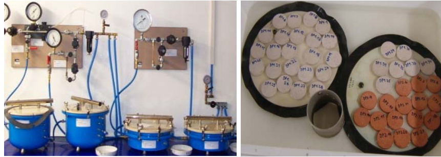
Figure 3-5 Pressure plate extractor (left) and porous ceramic plate with specimens (right)
