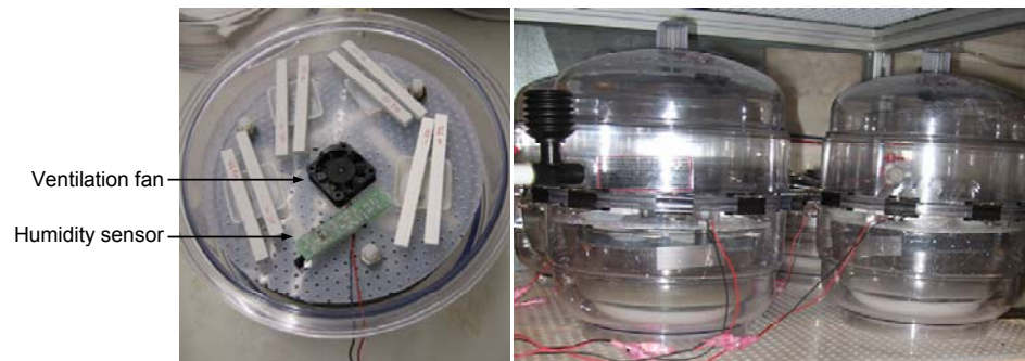
Figure 3-4 Desiccator chambers with the saturated salt-in-water solution
