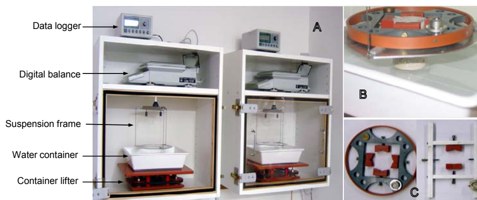
Figure 3-8 Automated water absorption apparatus (A); specimen fixed in specimen holder hanging above the water by suspension frame (B); different types of specimen holders (C)
