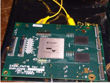
Fig. 3. Va_MaPMT ASICs mounted on the hybrids used in the BTeV gas RICH prototype studied with test beam runs at Fermilab.
