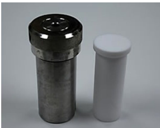
Figure 2.3. Autoclave and Teflon liner for hydrothermal synthesis. 118
