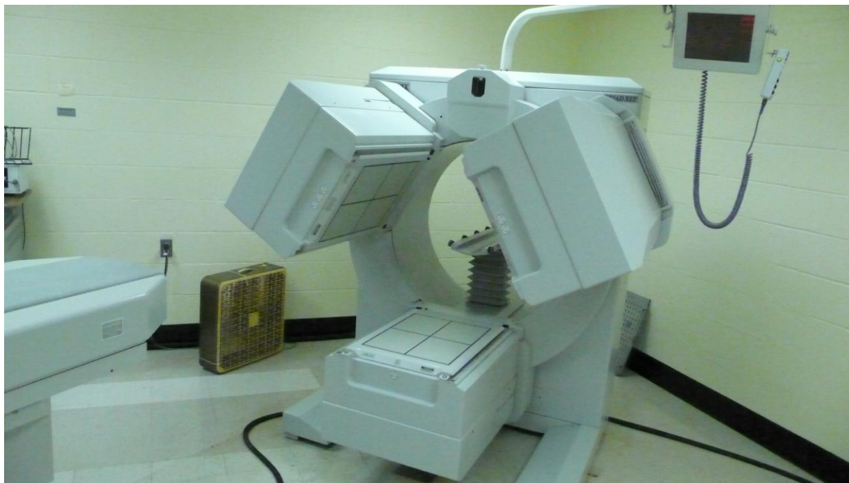
Figure 1.1. TRIAD XLT triple-head gamma camera (Trionix Research Laboratory, Inc., Twinsburg, OH) in use at SUNY Upstate Medical University (courtesy of SUNY Upstate Medical University).
