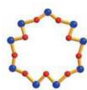
Figure 5.3. A ball-and-stick representation of the \{\text{Mo}_9\text{O}_9\} pore present in Mo-132. Blue spheres – molybdenum; red spheres – oxygen. 21
