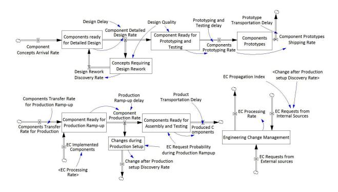
Figure 25: The Model Template for Supplier involved in Design and Manufacturing phases
