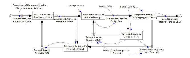
Figure 27: The Model Template for Supplier involved in Concept and Design phases
