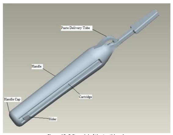
Figure 13: 3-D model of the toothbrush
