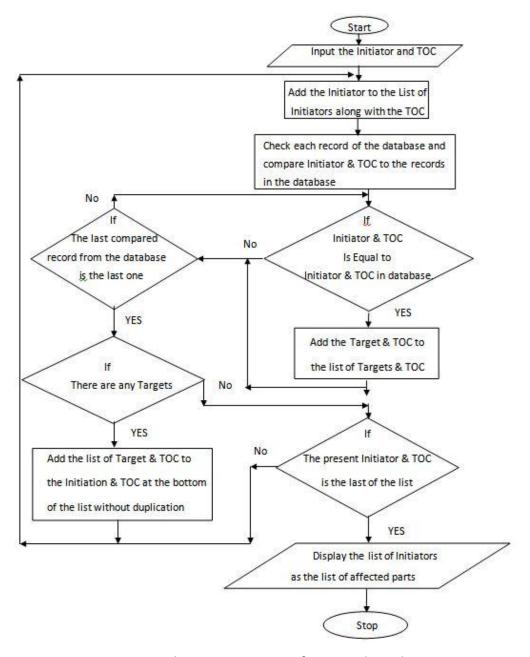
Figure 11: Change Propagation framework Implementation Logic
