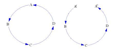
$$Polarity = SGN\left(\frac{\partial A^O}{\partial A^I}\right)$$
