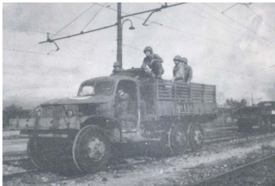
Figure 27: Truck Reconfigured as Rail Engine 652
