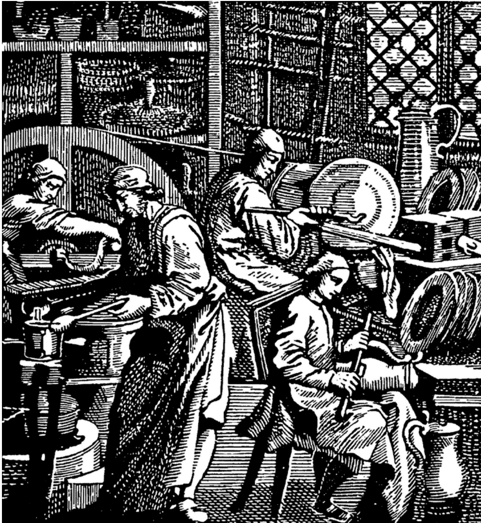
Figure 4.10 Der Kandelgiesser (The Pewterer), a copper engraving by P. Abraham and S. Clara, Würzburg, Germany, 1699. The craftsman in the background is producing spun hollowares on a flywheel driven lathe (Barkin 1988:8).
