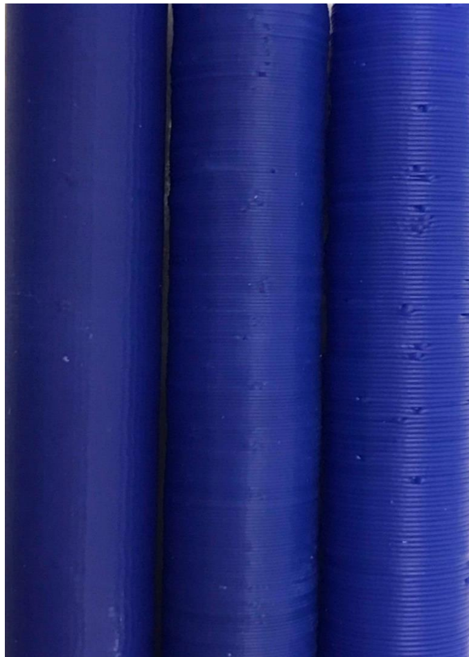
Figure 1. Direction of the acetone smoothing and sanding treatments.
