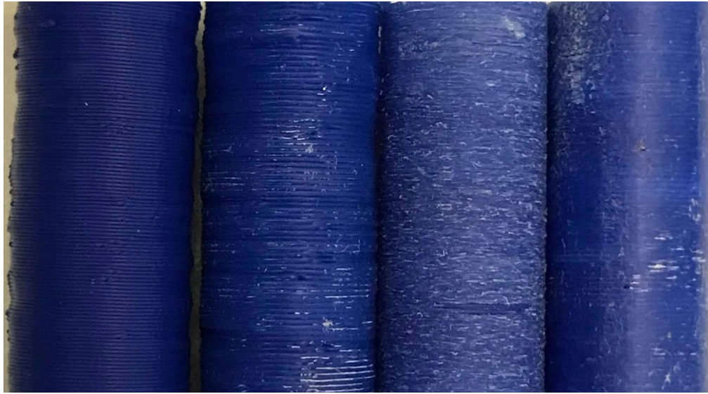
Figure 3. 3d Printed ABS tube with 0.3mm layer height and surface treatments applied – (From left to right) No surface treatment, rubbed acetone treatment, sanding, and sanding followed by rubbed acetone treatment.
