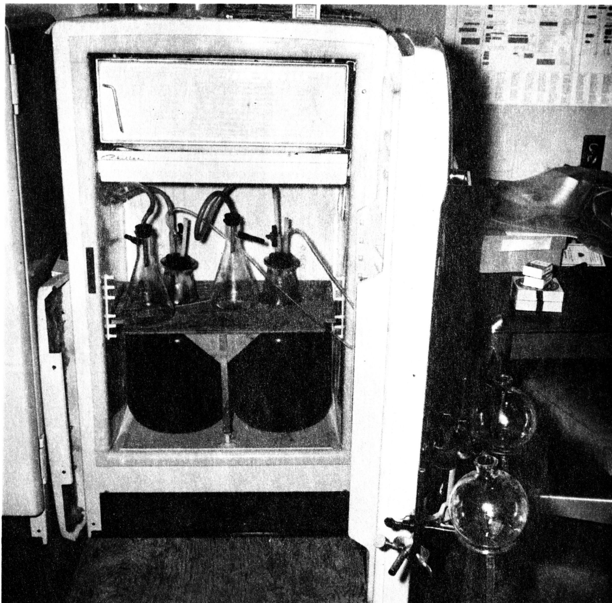
FIGURE 5. DIGESTION EQUIPMENT AT 5°C. NOTICE SMALL GASOMETERS USED.
