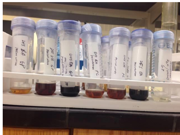
Figure 3.23. Liquid-liquid extract of piperine in ethyl acetate.
