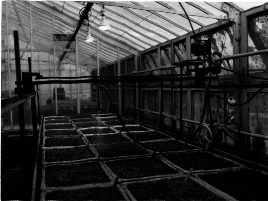
Figure 1. A Greenhouse Experiment Showing the Simulated Rainfall Applicator in Operation
