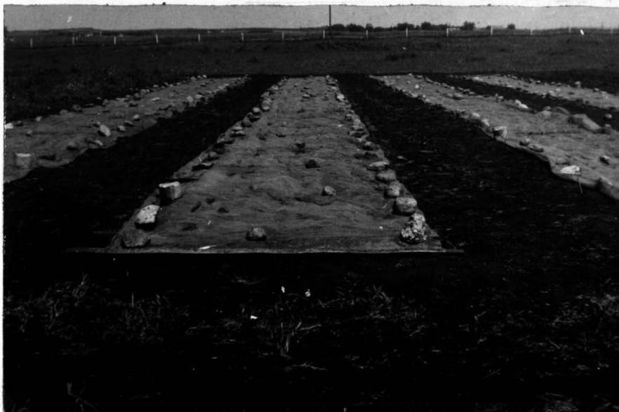
Figure 5. Field Plots Covered with a Four-mil Polyethylene Plastic Sheet Just After a Rain
