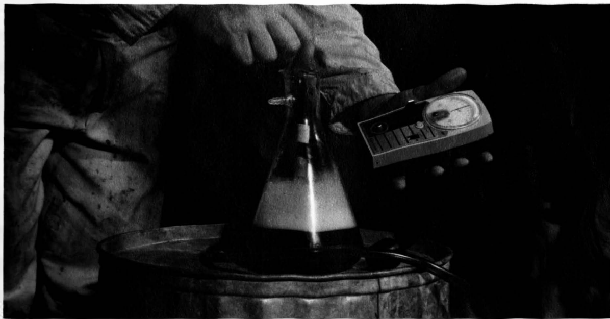
Figure 2. A view of the determination of pH using a portable pH meter.
