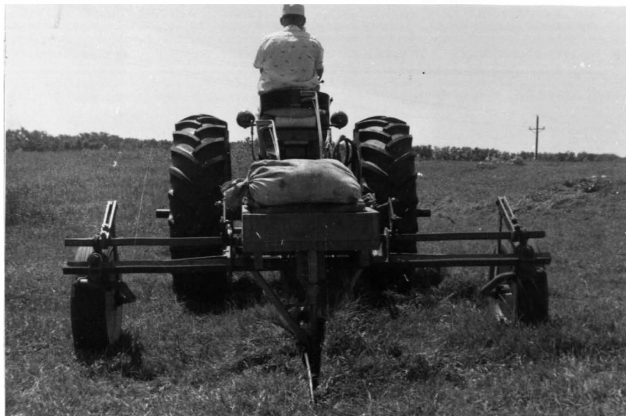
Figure 22. Pasture Furrower in Operation
