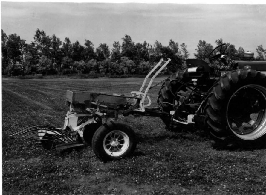
Figure 7. General View of the Pasture Furrowing Machine with Box Provided for Accommodating the Addition of Extra Weight
