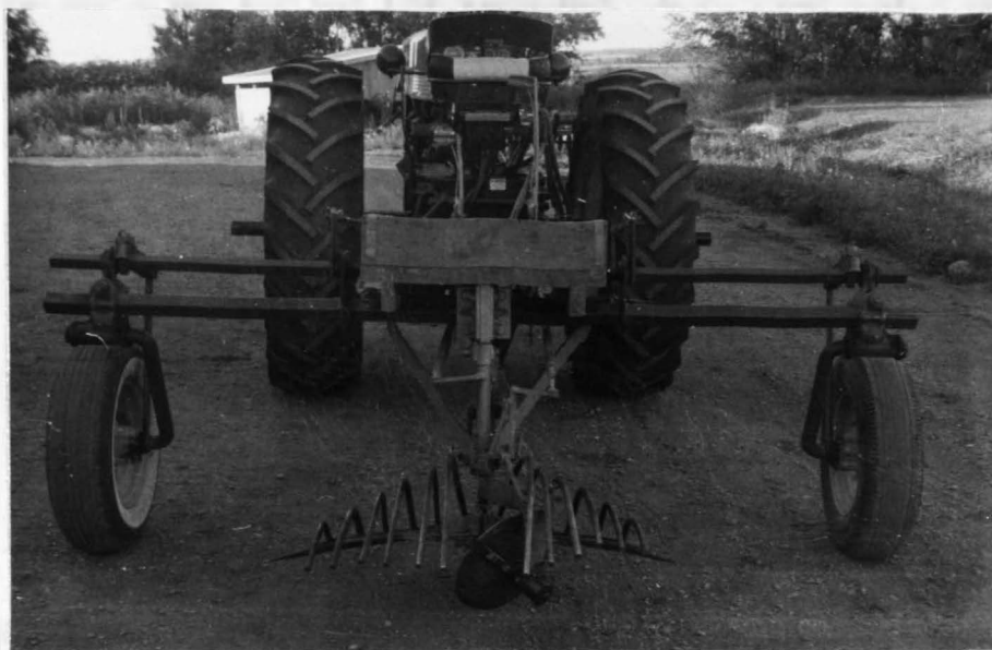
Figure 10. Rear View of Pasture Furrower Showing Lateral Slope of the Sod Rack
