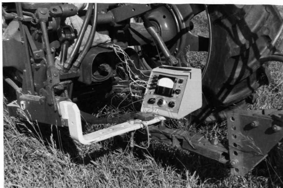
Figure 21. Strain-Gage Transducer and Amplifier Mounted on the Tractor Drawbar
