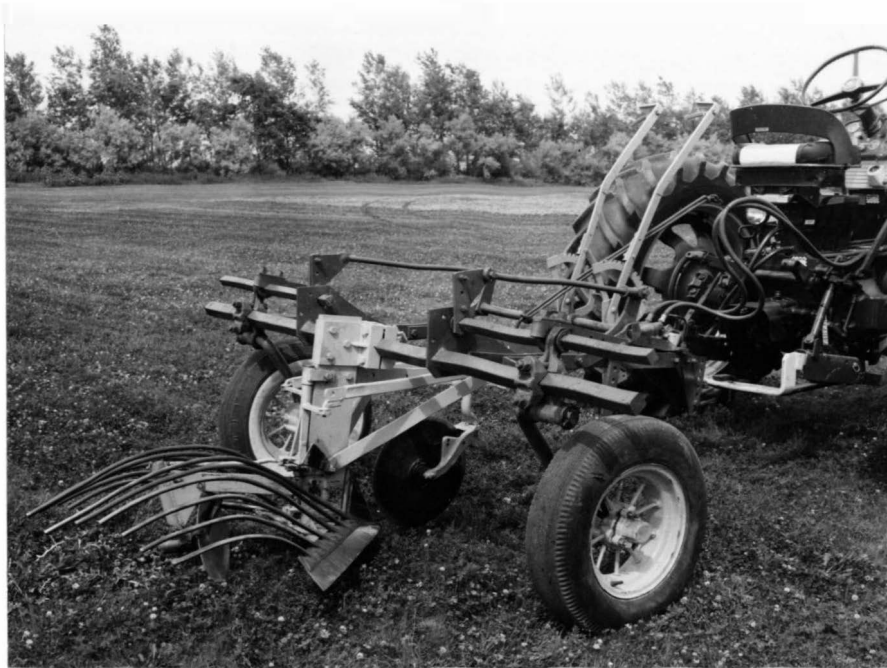
Figure 6. General View of the Pasture Furrowing Machine
