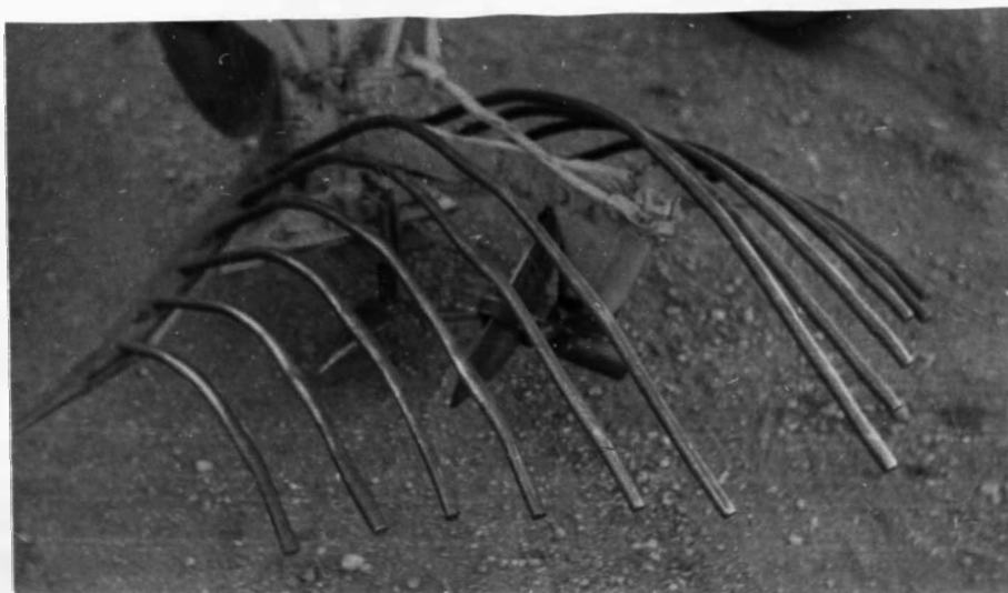
Figure 20. Straight and Sweep Type Scarifying Blades Attached to the Furrower
