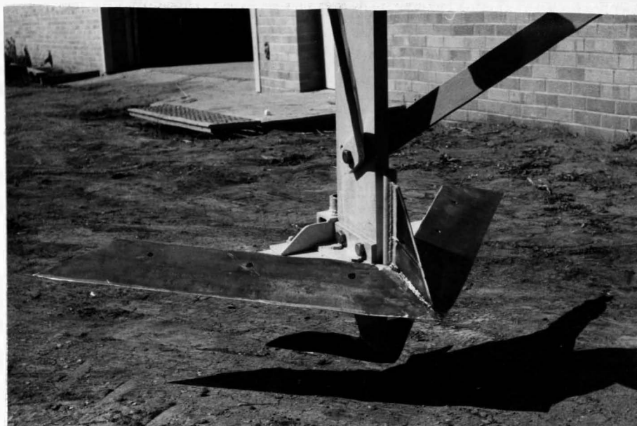
Figure 9. Relative Location of the Vertical Knife on the V-Blade
