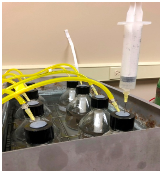
Figure 7. Withdrawing the headspace gas from the test bottle
