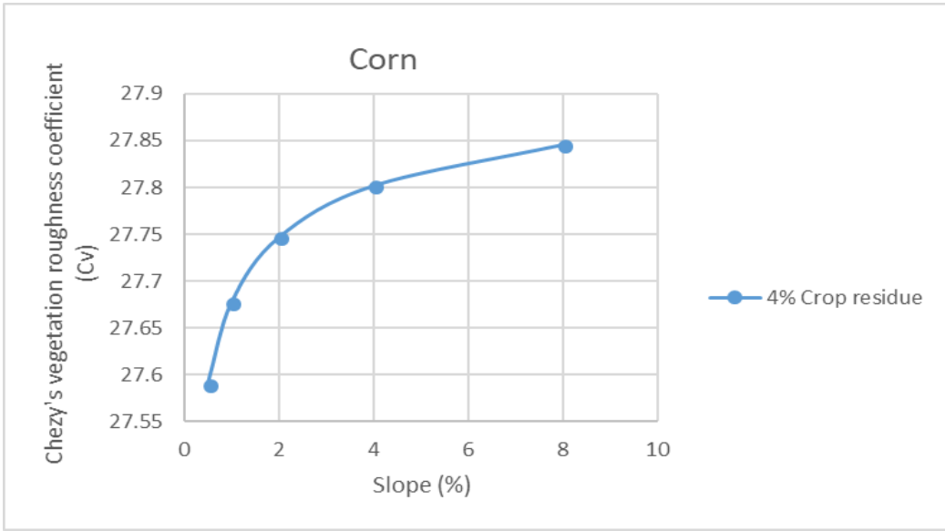
Figure 4.8 Chezy's vegetation roughness values based on slope
