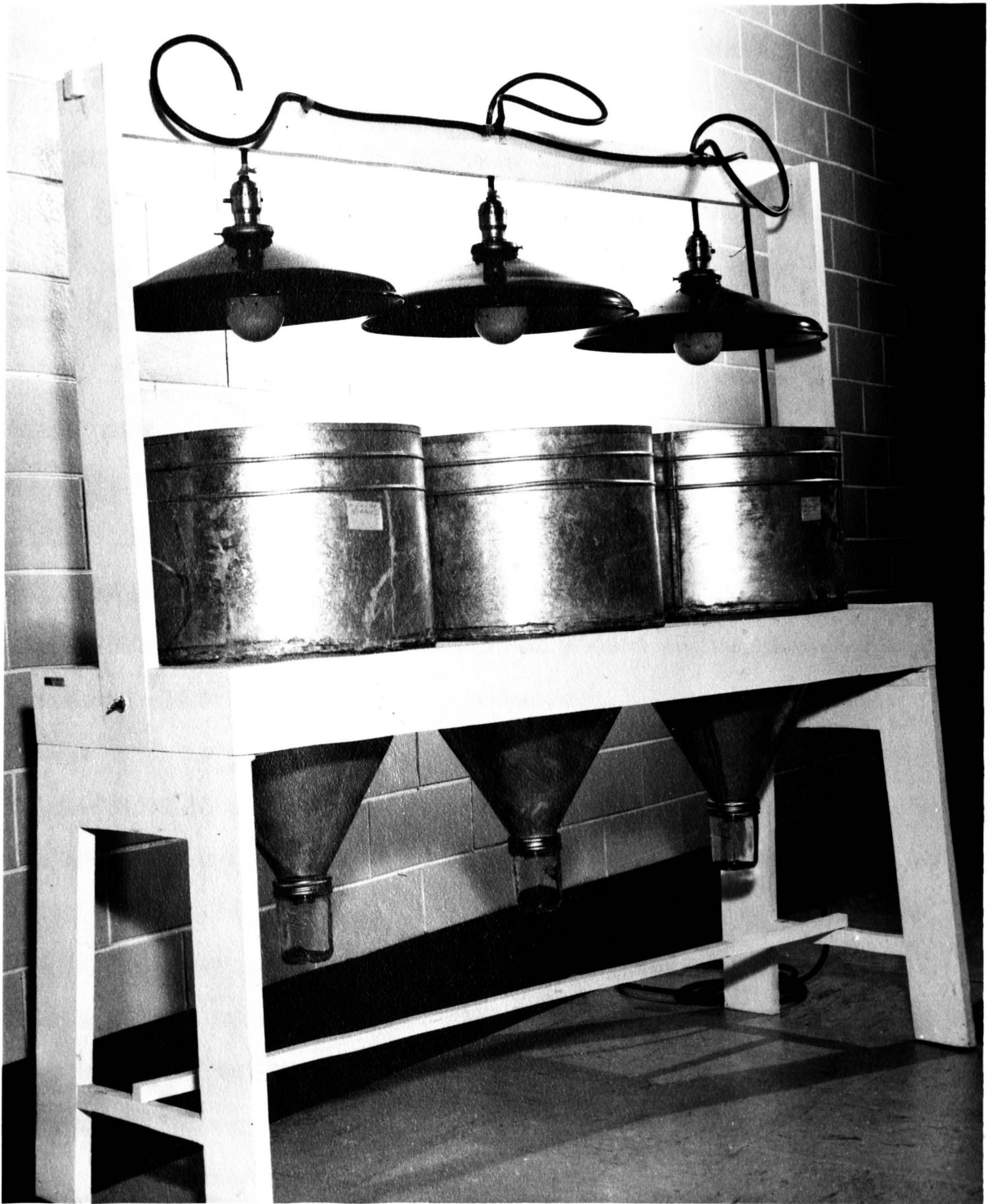
FIGURE 5. BERLESE TYPE FUNNEL BATTERY
