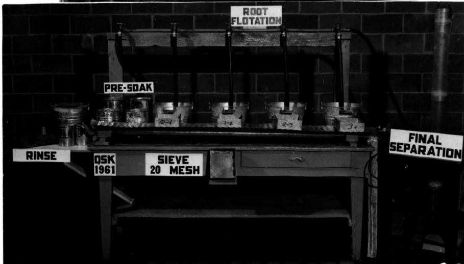
Figure VI. The apparatus used for separation of the corn roots from the soil
