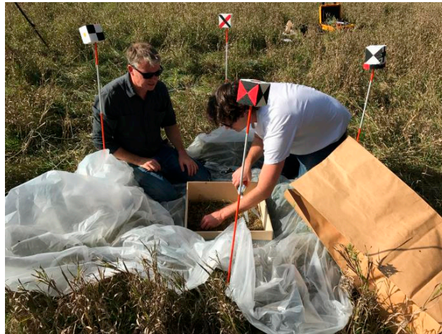
Figure 1. Destructive harvesting of the aboveground grass biomass in 1 of the 11 grass plots. Note that the four poles are not vertical in this picture as the harvesting is undertaken after the remotely sensed measurements and so the poles have been pushed aside. The wooden frame is 0.46 m × 0.46 m and the four poles are 1.2 m tall (see text for details).
