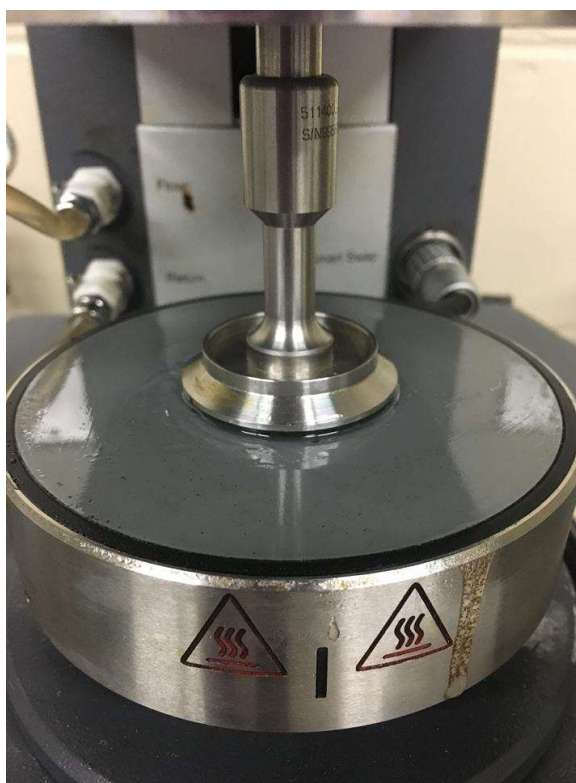
Figure 23. Rheological test being performed at a PGSA sample
