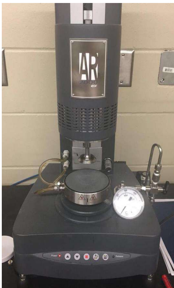
Figure 22. AR2000 Rheometer used to perform viscosity tests
