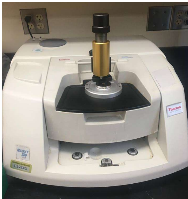
Figure 21. Machined used to perform FTIR tests
