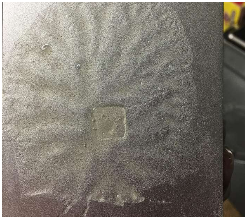
Figure 55. Primary tests of 3D printing PGSA proving that a thin layer of the material adheres to the building plate
