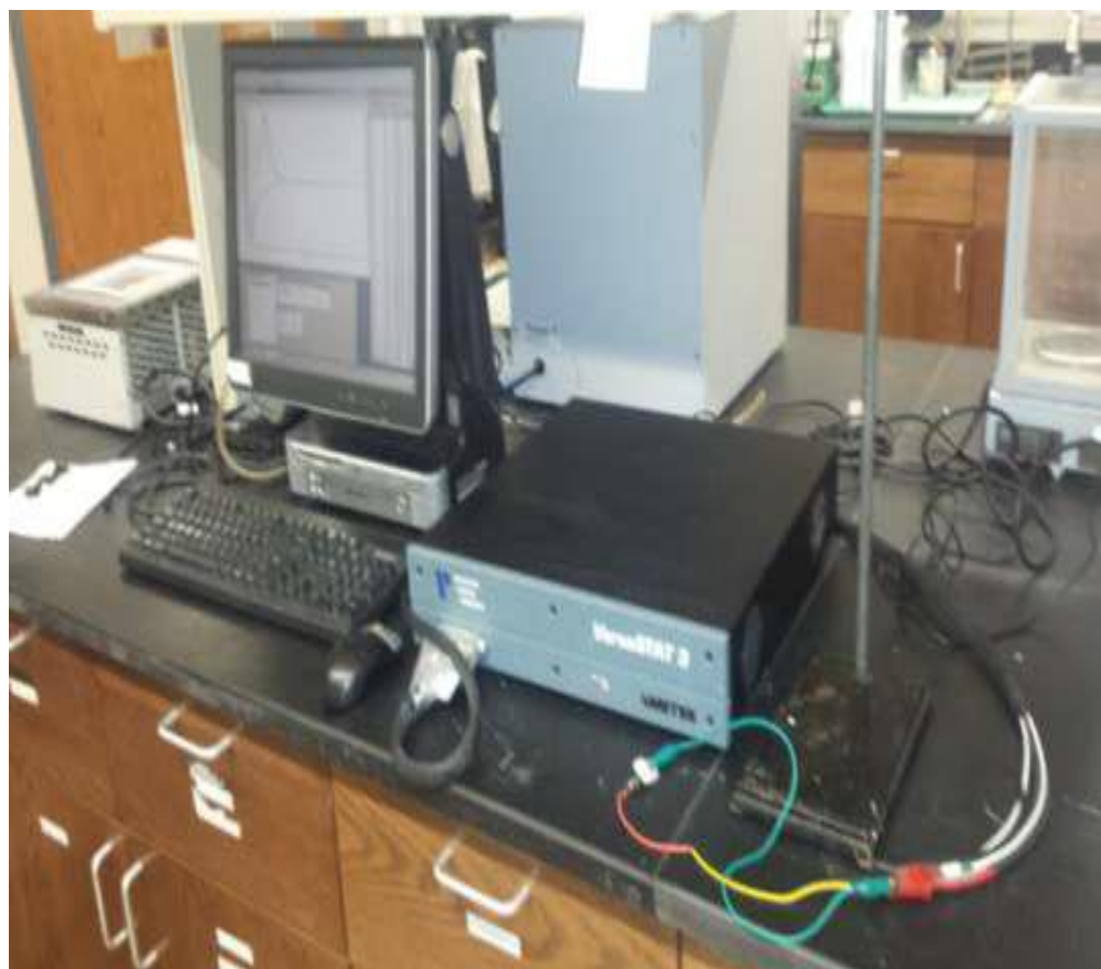
Figure 3.20: System setup used for Electrochemical Impedance (EIS) and Cyclic Voltammetry (CV) measurement
