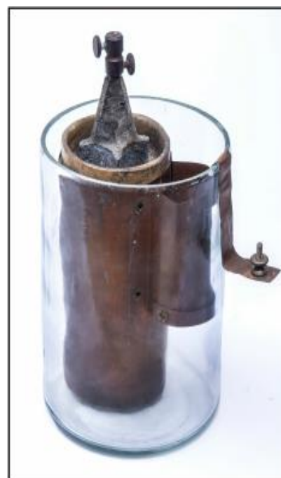
Figure 1.10 An actual surviving example of the Daniell cell (Jensen-Thomas Apparatus Collection) [10]
