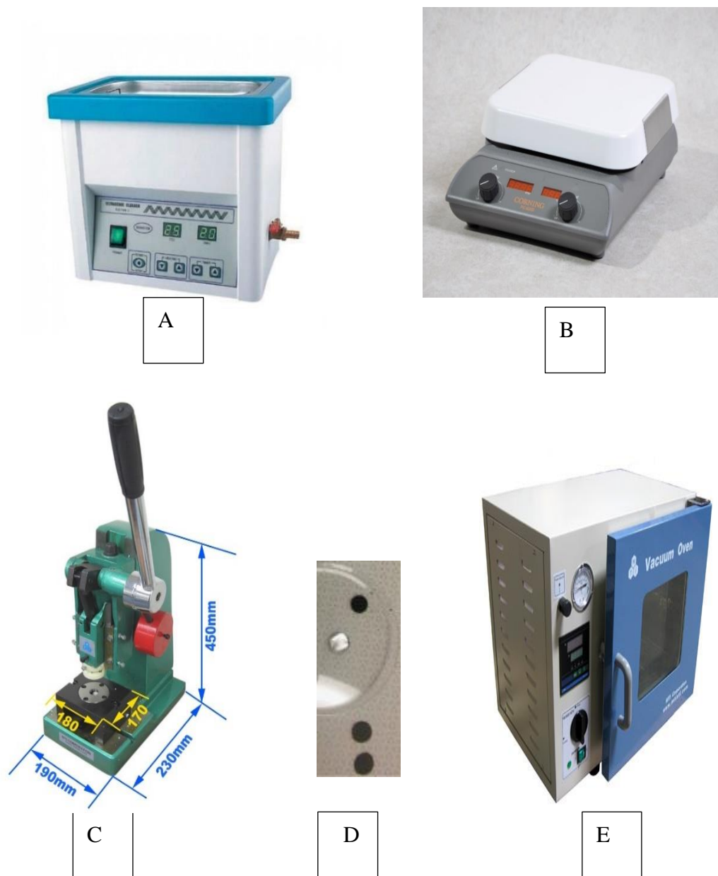
Figure 3.16. (a) Ultrasonicator (b) Hotplate, (c) Disc Cutter, (d) Sample, and (e) Vacuum Oven
