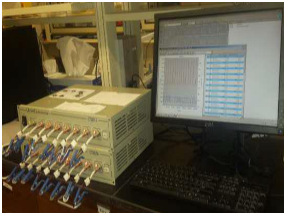
Figure 3.19: LAND CT2001A battery Analyzer system setup.
