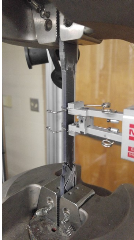
Figure 3-4: Mechanical testing of 3D printed specimen using an MTS 858 universal Testing Machine
