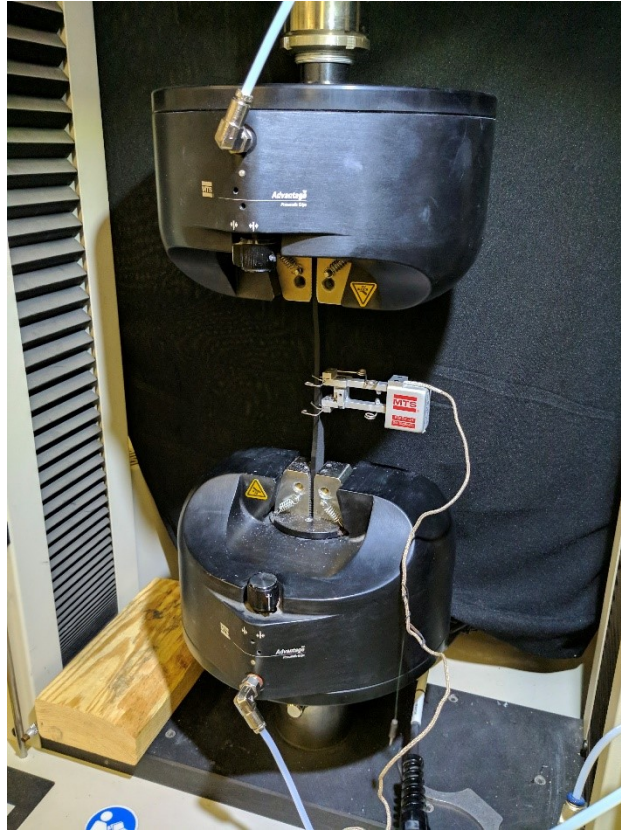
Figure 2-5: Mechanical Testing of 3D printed specimen using an MTS Insight Tensile Testing Machine
