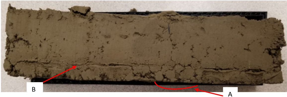
Figure 4.2.2. Flexural cracks on the extracted clay sample.
