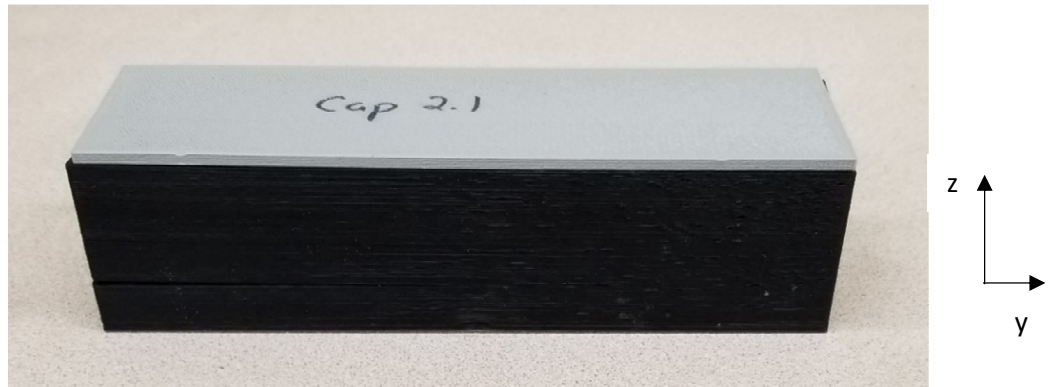
Figure 3.2.5. The first assembled CT beam.
