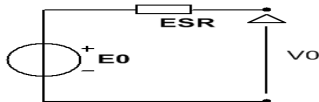
Figure 2. 3: Simple battery model [25].
