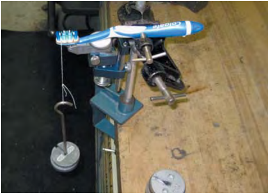
Figure 7. Measuring Spring Constant of Head and Neck
