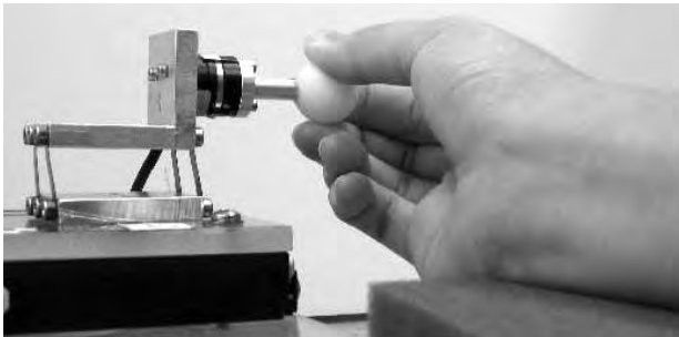
Figure 5. Hand Vibrational Properties Measuring Apparatus [3]
