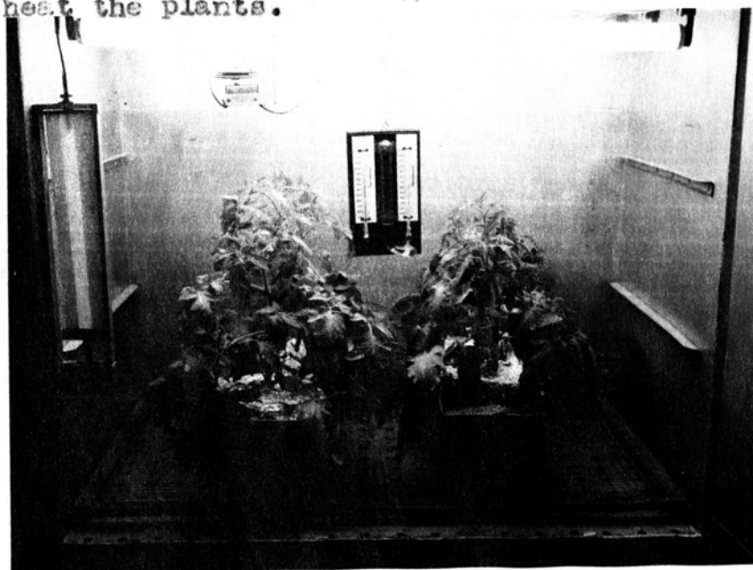
Fig. 2. The chamber (Fig. 1) is equipped with three daylight bulbs of about 200-225 foot candles
