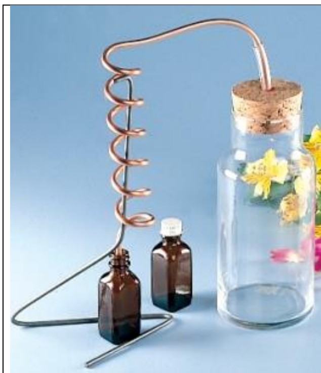
Figure 1: Perfume distiller set-up for final extraction but not showing the lard. The arrangement shown was formerly available from Scientificsonline.com as part of a kit.
