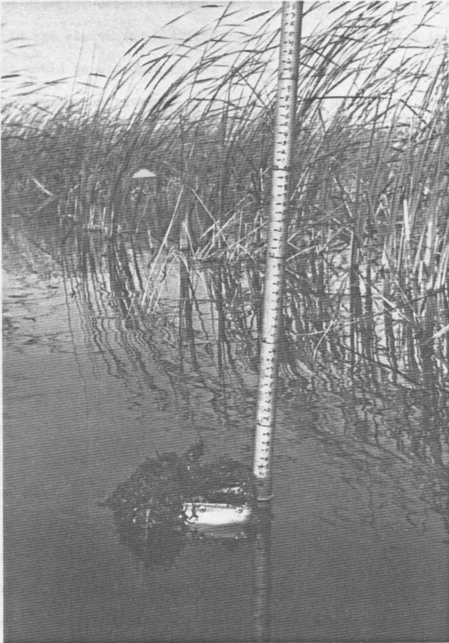
Figure 2. A sampler used to collect quantitative samples of aquatic plant communities and associated invertebrates.
