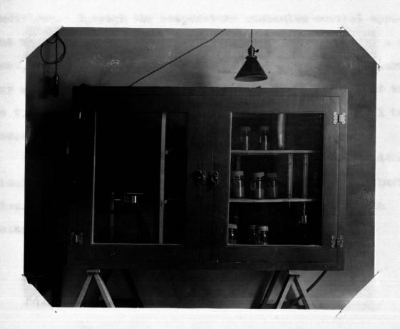
PLATE I. - Photograph showing cabinet and arrangement of apparatus used in controlling temperature and relative humidities during the investigation.
