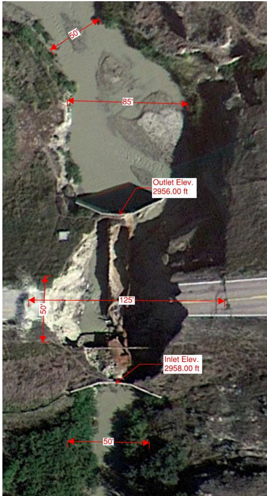
Figure 3.7: 12 foot CMP culvert with estimated dimensions (Google Earth, 2015)
