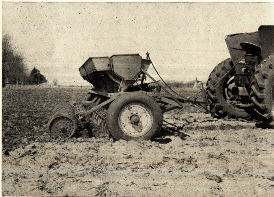
Fig. 1. A combination grain-fertilizer drill is the most effective method of applying fertilizer to small grains.
