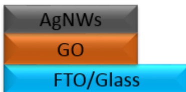
Figure 3. 4 Layer by layer electrode of GO/AgNWs.
