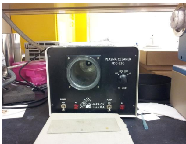
Figure 3. 2 Picture of oxygen plasma cleaner.
