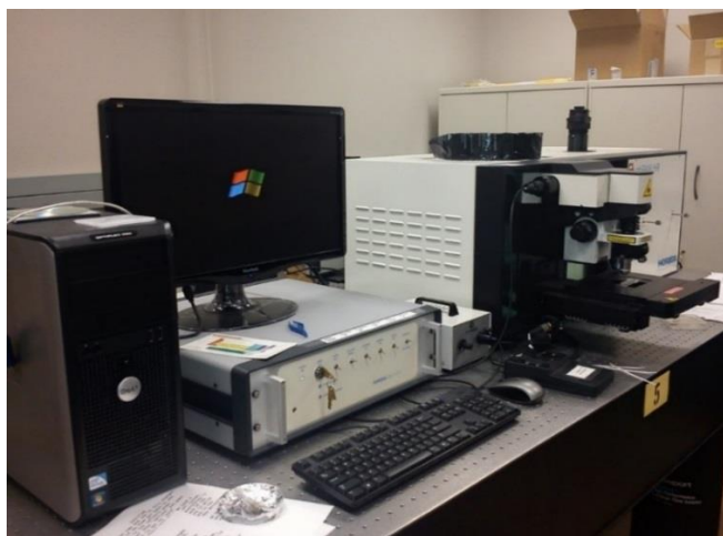
Figure 3. 7 Photograph of the LabRAM HR Raman spectroscopy.
