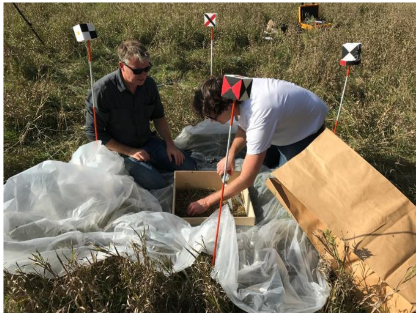
Figure 2. Destructive sampling of aboveground grass biomass in one of the grassland plots. The four poles roughly delineate the 1 x 1 m plot and were used as reference points for aligning the SfM and TLS point clouds.
