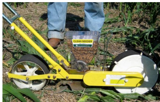
Figure 2-5: The single-row push drill used for drill cover crop interseeding procedure.
