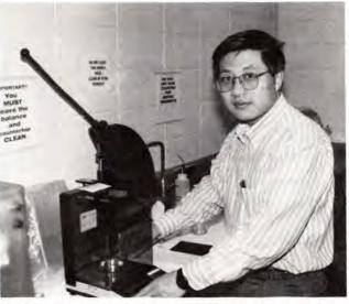
Dr. C. Y. Wang uses an electronic balance to accurately weigh a sample of soy flour. The material is the basis for soy isolate, which is 90 percent protein.
