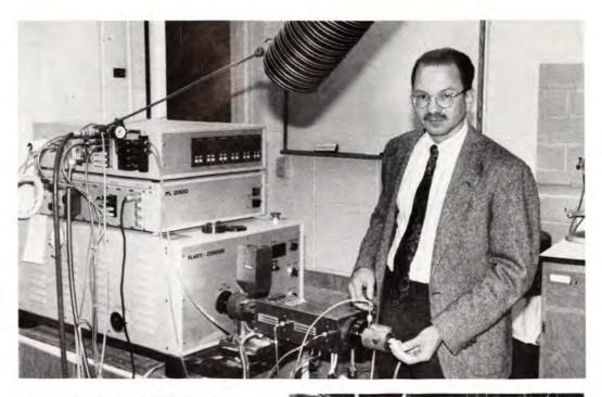
Jim Julson of the Ag Engineering Department demonstrates the lab-sized extruder used in SDSU's biodegradable plastics research. Plastic material coming from the extruder resembles corn curls. The extrusion process creates air cells in the material to enhance its shockabsorbing and insulative properties. Now that the team's formulation for the material is close to the optimum, it will be tested further through a commercial-sized extruder at a manufacturing plant in Minneapolis.
