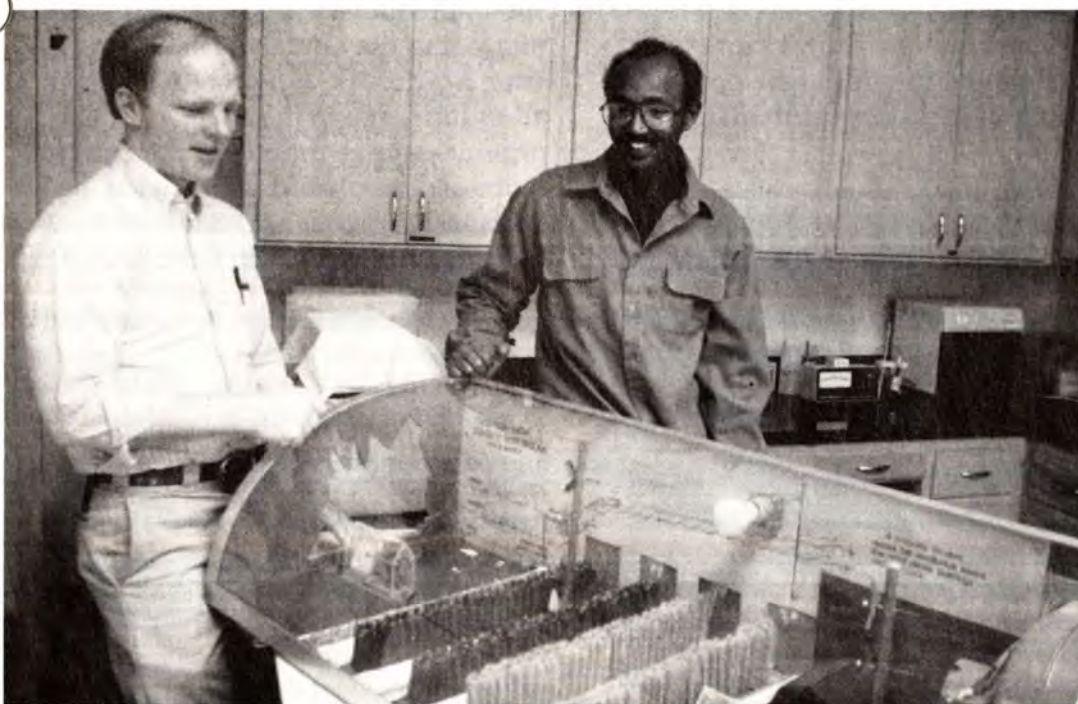
Pete Schaefer, left, can dispel doubts about the ability of a windbreak to slow down wind and snow by introducing smoke at different velocities at the end of this wind tunnel constructed in the Horticulture Forestry Department. Watching is Ismail Ahmed, also of the Horticulture Forestry Department.
