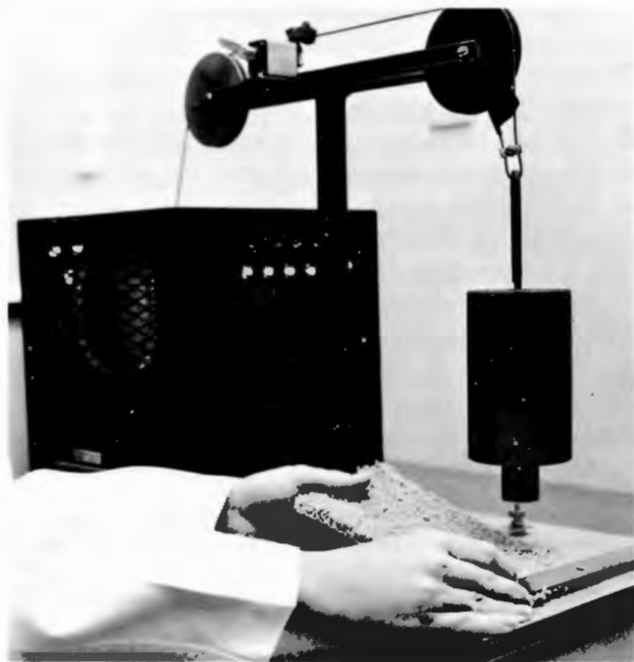
A device designed and constructed by State University engineers for use in textile research to measure the effects of crushing pressure on carpets.
