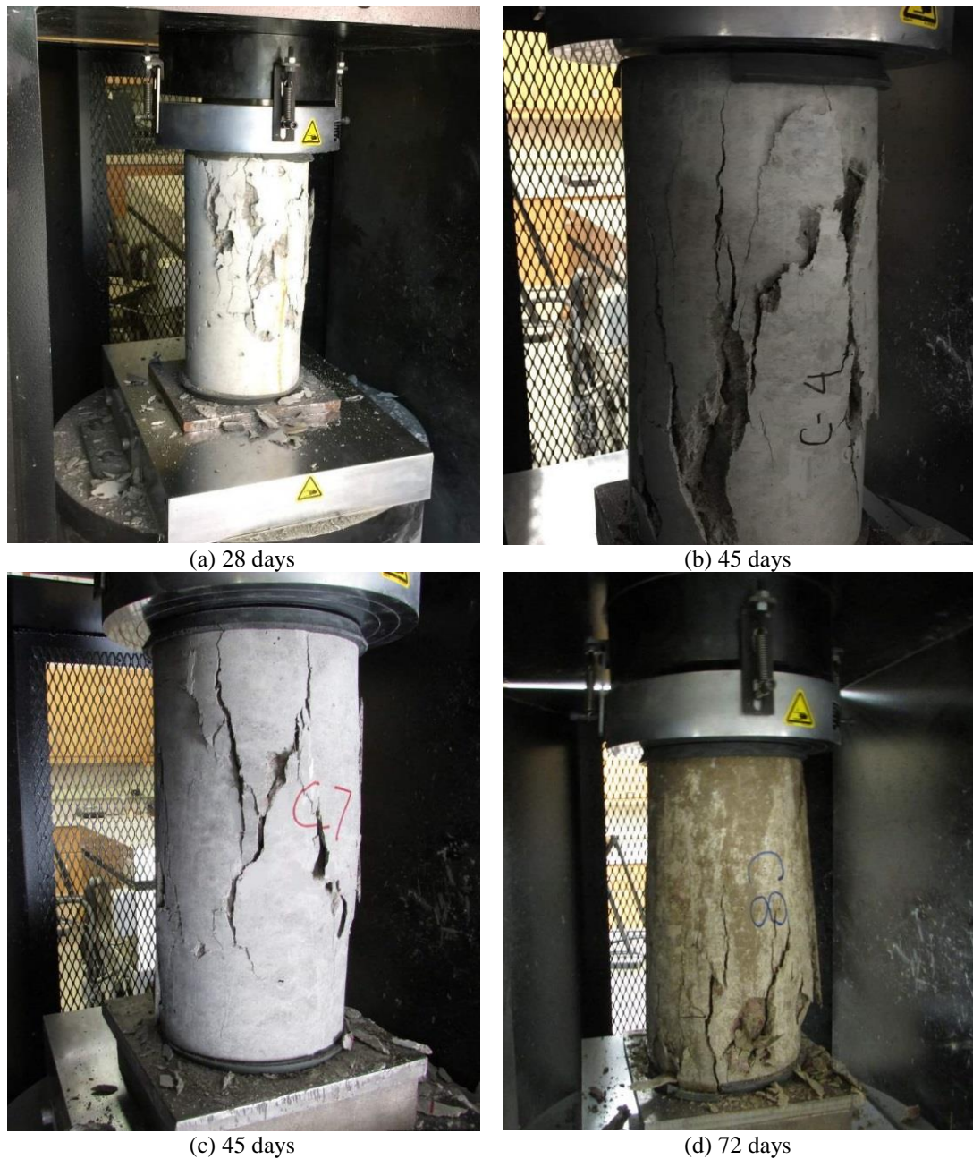
Figure 2-14. Failure of unconfined concrete specimens at different ages
