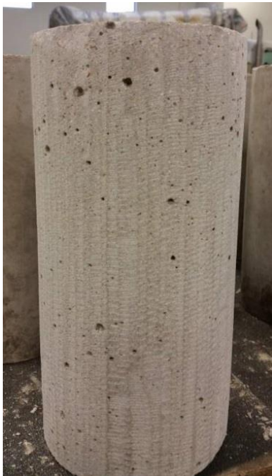
Figure 2-6. Concrete surface preparation for two specimens
