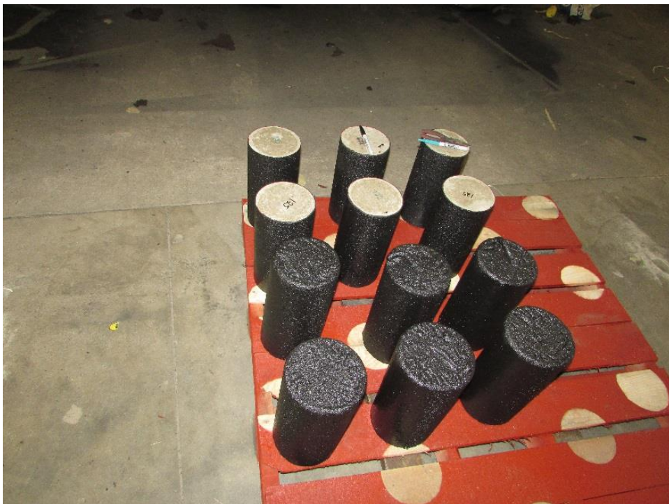
Figure 2-10. Rubber-coated concrete specimens
