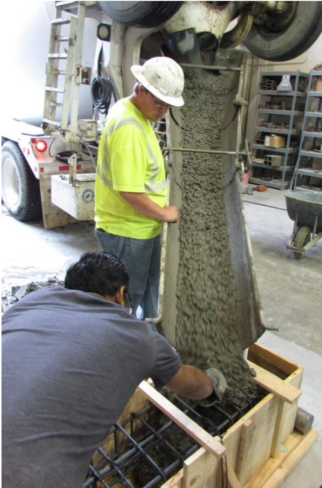
Figure 4-18. Concrete pouring for beam-column test specimen
