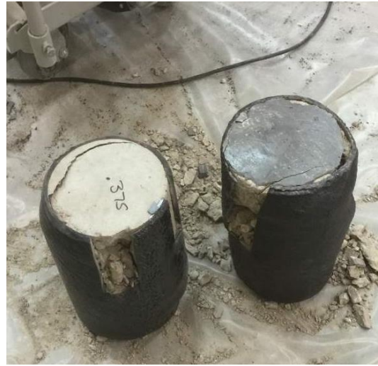
(b) Extracting Rubber to determine thickness
