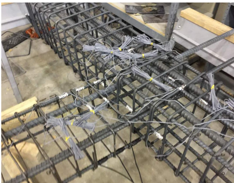
Figure 4-25. Installation of strain gauges in beam-column specimen
