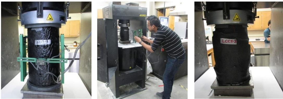
(a) Damage at maximum stress (strain 0.001791 in./in.)
