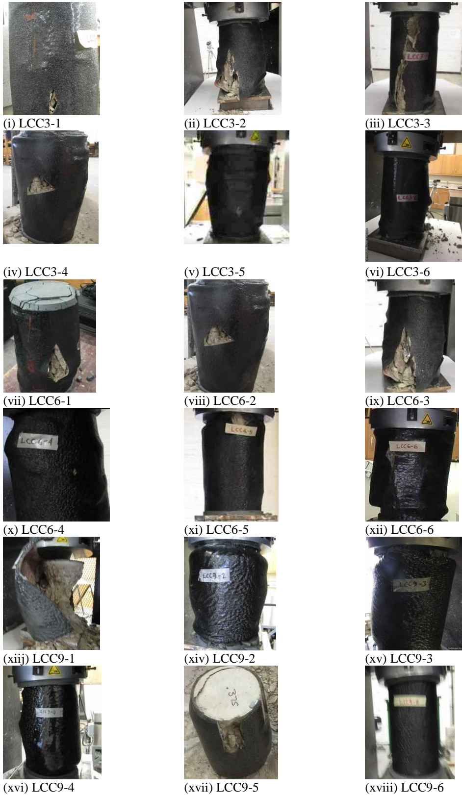
Figure 2-20. Failure of all rubber confined concrete specimens
