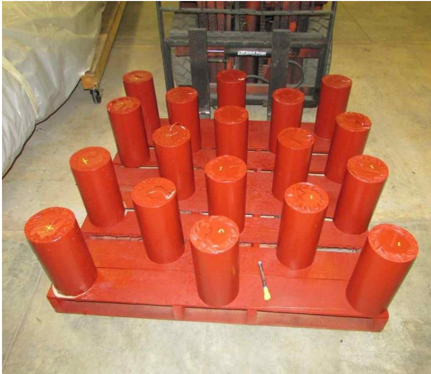
Figure 2-7. Thin layer of base coat on concrete
