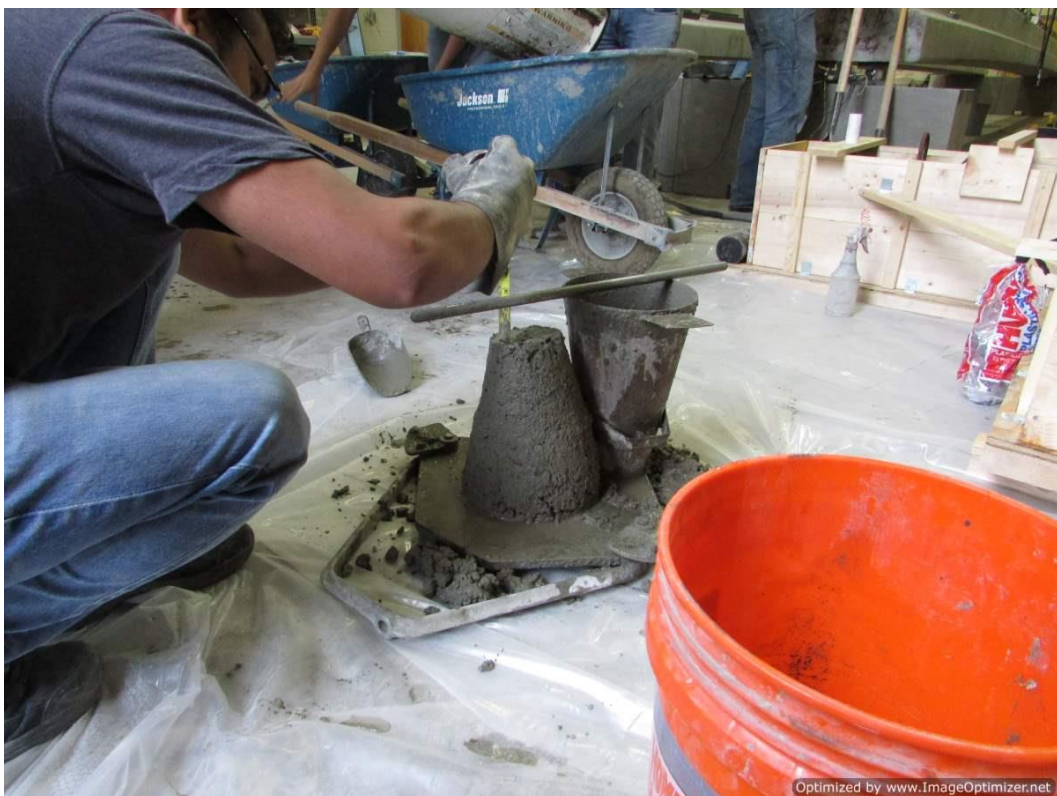
Figure 4-17. Slump of ready mix concrete
