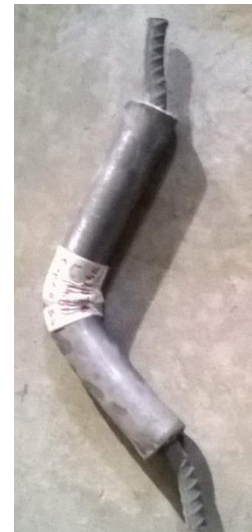
(b) BRR device at failure
