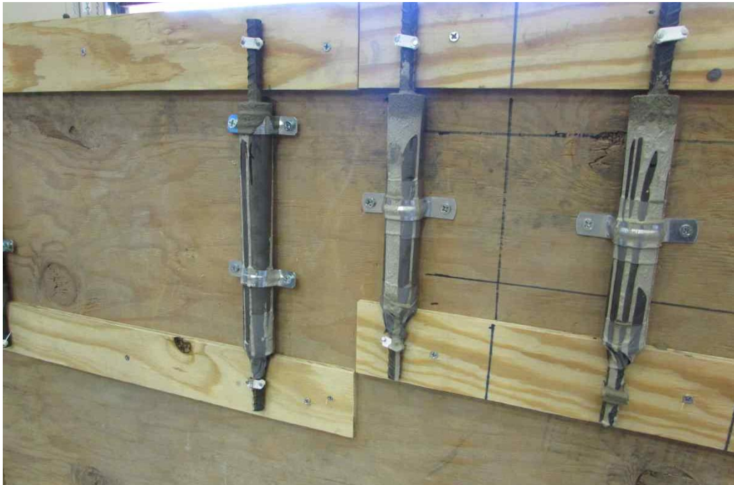
Figure 3-14. BRR specimens after pouring non-shrink grout
