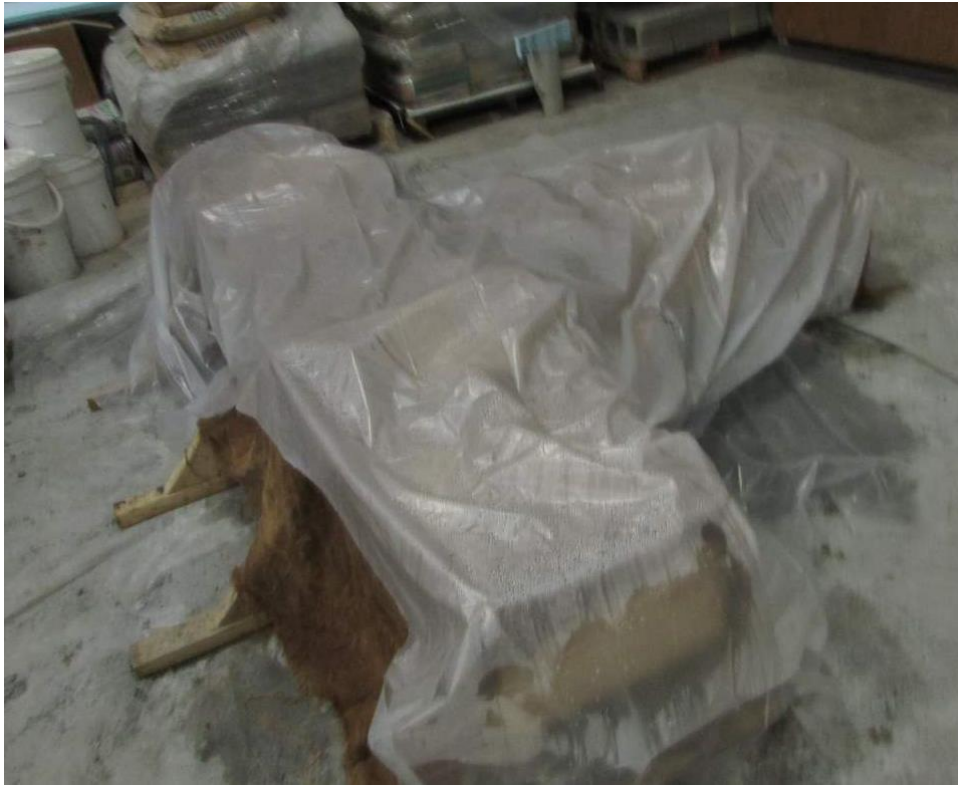
Figure 4-19. Curing of beam-column test specimen
