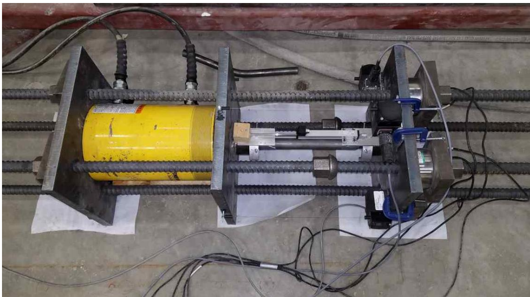
Figure3-16. Photograph of BRR test setup
