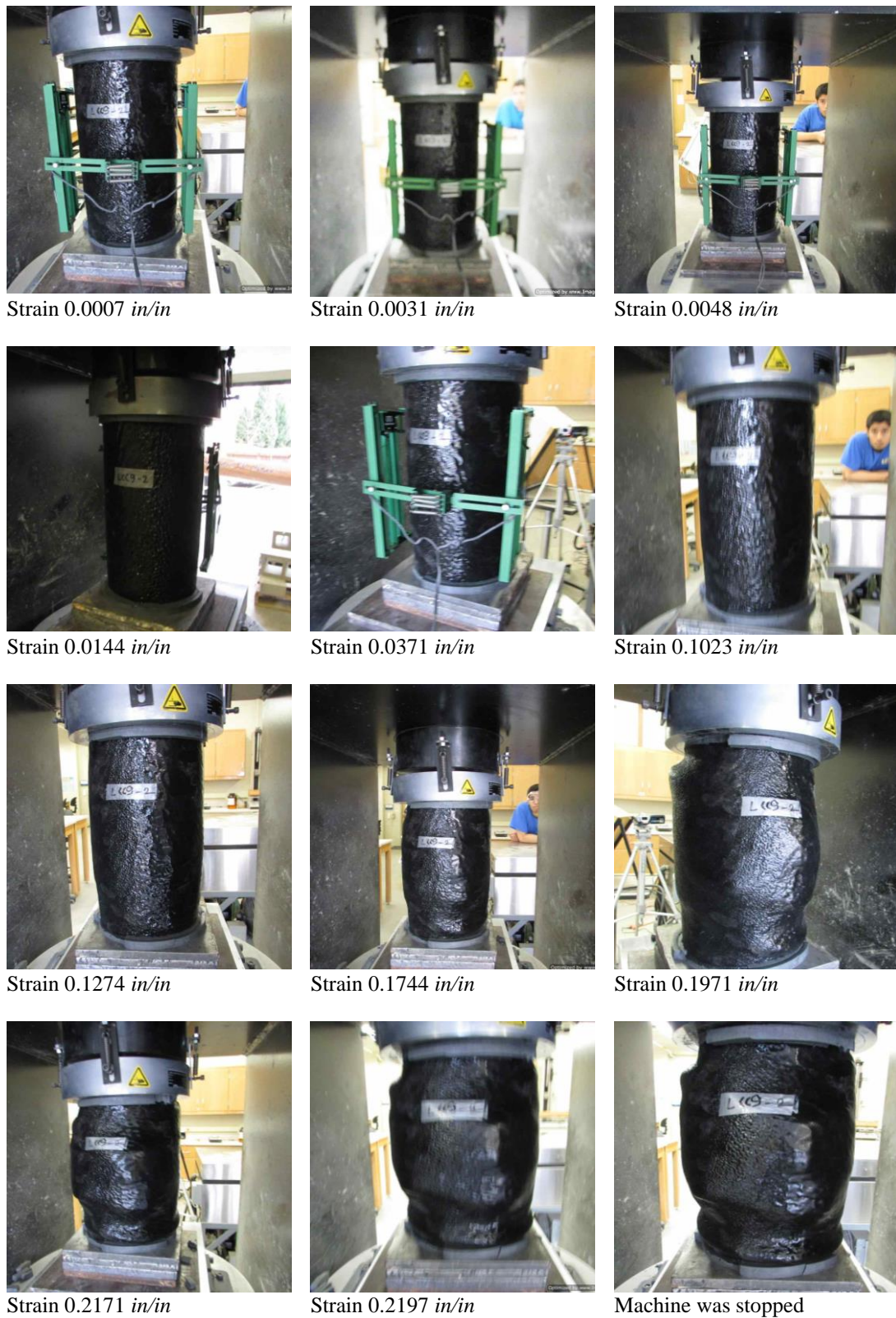
Figure 2-22. Strain capacity of rubber confined concrete at different stages during uniaxial compression test: Specimen LCC9-2
