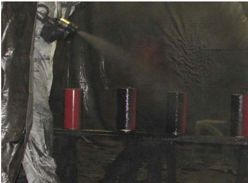
Figure 2-8. Spraying rubber on concrete specimens
