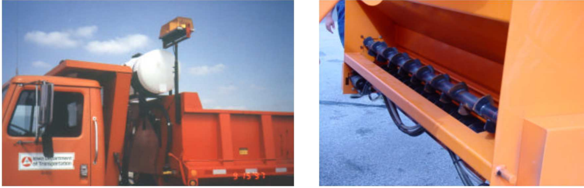
Figure 2.2 A typical truck with a brine pre-wetting unit (left) and a truck with an auger used to break up any salt clumps that may form (right) (Iowa DOT).
