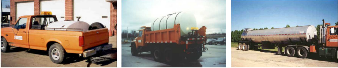
Figure 2.3 Brine spreading trucks, 250 gallons (left), 1,800 gallons (middle) and a 5,000 gallons (right) (Iowa DOT)
