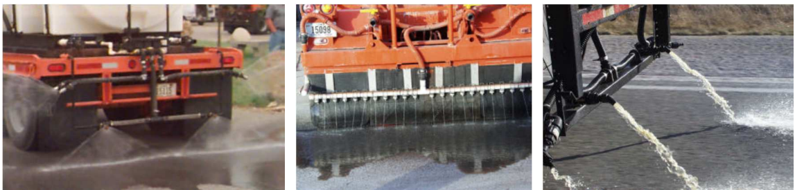
Figure 2.4 Brine spreading nozzles, fan style (left), streamer nozzle (middle) and concentrated method (right) (Iowa DOT)
