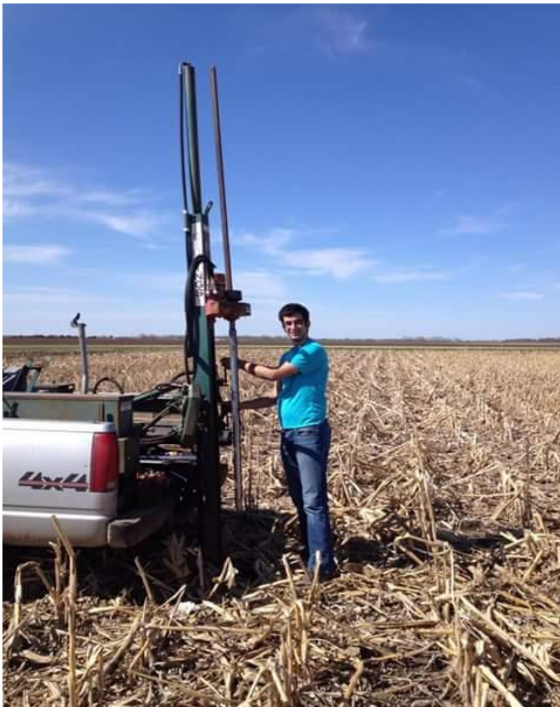
Figure A4.6. Taking soil samples from field to analyze soil properties such as SOC, TN, pH, EC and WAS.
