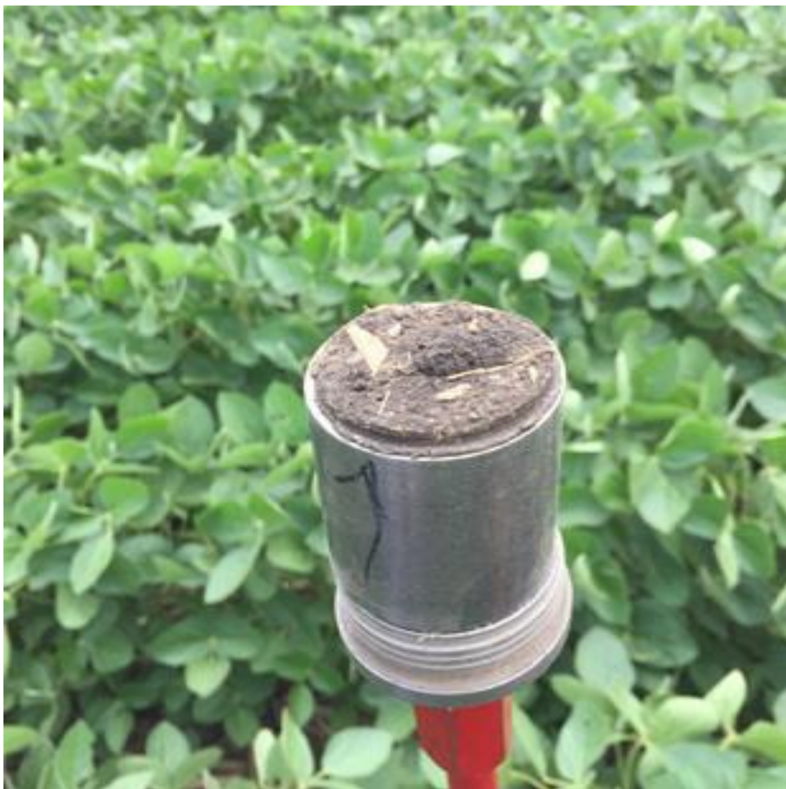
Figure A4.7. Taking core samples from field to analyze bulk density, soil water retention and pore size distribution of soil.
