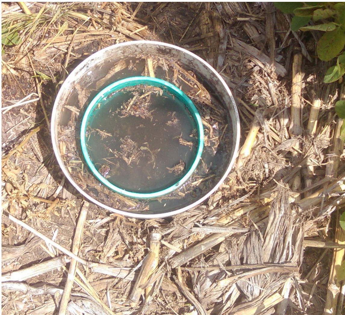
Figure A4.8. Examination of water infiltration rate in the field by using double rings method.
