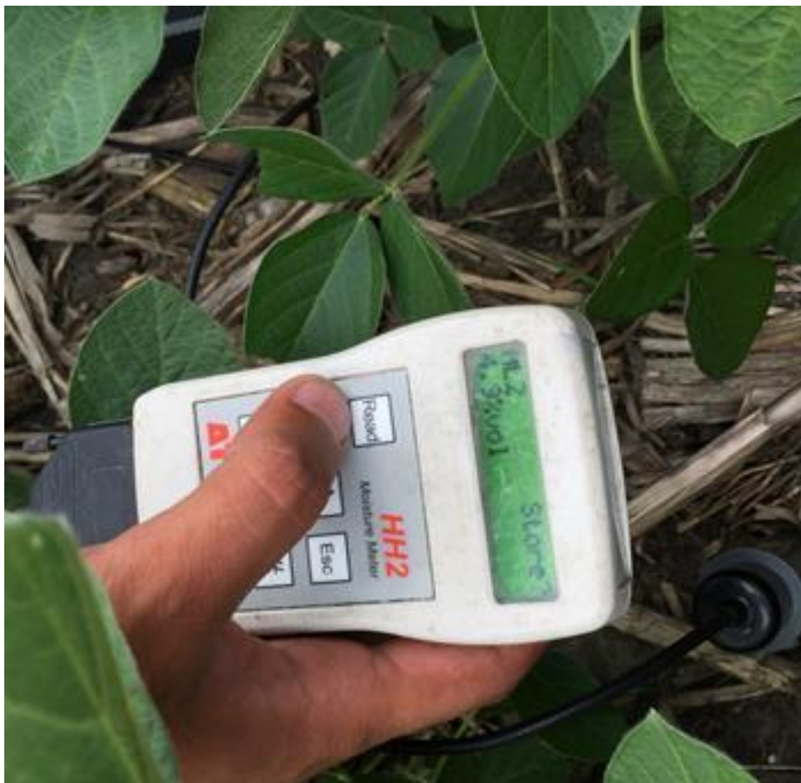
Figure A4.12. Taking volumetric soil moisture readings from field.
